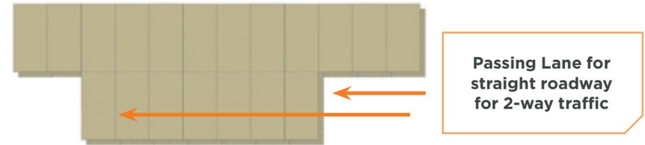
While straight roadways are ideal, there will always be situations where the length of the roadway would dictate the need for a passing area. For these situations, it is possible to add additional mats to the roadway for both the short-side and long-side connection methodologies.
